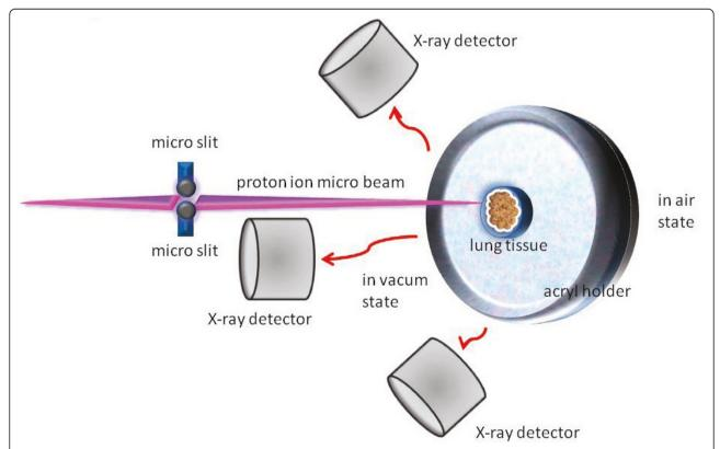
**Figure 1 In-air micro-PIXE system**. The proton ionmicrobeam from the accelerator is focused through microslit, and the beam is irradiated to the tissue sample in vacum state. The characteristic X-rays, those are specific energy for each element produced by irradiation, are identified by the X-ray detectors.
